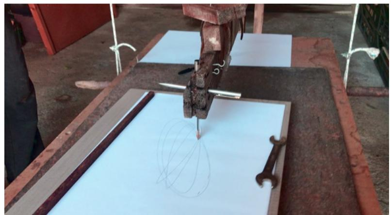
Kamil Arčon invented and constructed a variant of mechanical pendulum "NIHALOPIS", which he used to graphically explore the beauty of the world of symmetries. Fascinated by complex motion of Nihalopis, which represents an interesting example of a coupled pendulum, he systematically charted a series of different trajectories and modes of motion, without any mathematical or physical knowledge.
