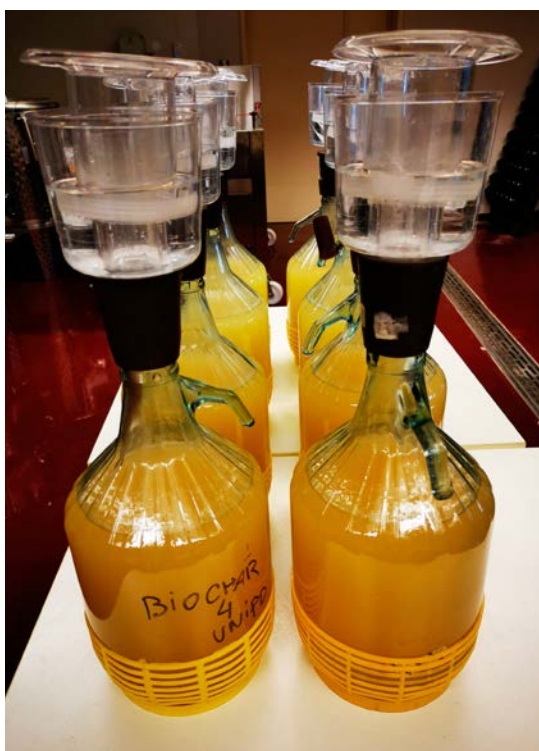
Microfermentations of grape must in the framework of a PhD thesis of a guest student from the University of Padua.
