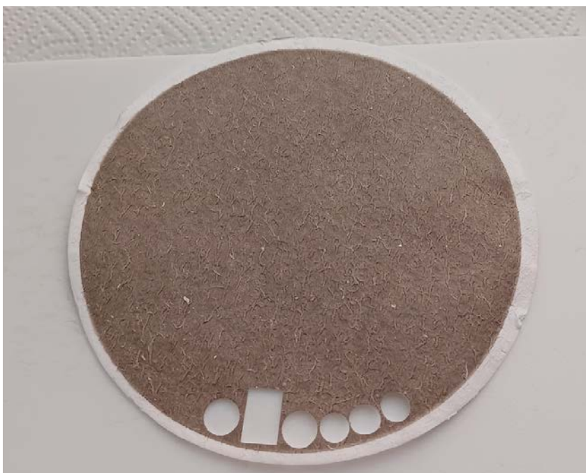
A filter sample loaded with PM 10 air particles, sampled at the Loka stream, being prepared for oxidative potential measurement.
