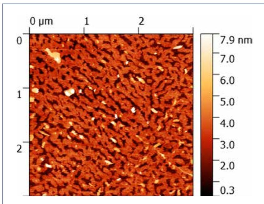
3x3 μm<sup>2</sup> atomic force microscopy topography image of graphene flake covered with high-carrier-mobility organic semiconductor, using molecular-beam epitaxy. Brighter tones represent higher elevations. The effective coverage is one molecular layer with a second layer in the nucleation phase (bright features).
