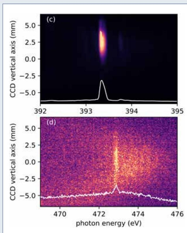
Coherent harmonic emission spectra of the FERMI FEL working in the EEHG configuration at (top) 3.1 nm (394 eV) and (bottom) 2.6 nm (474 eV).
