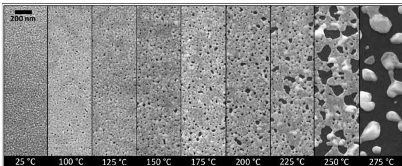
Temperature evolution of the Au film on the Bi<sub>2</sub>Se<sub>3</sub> substrate.
