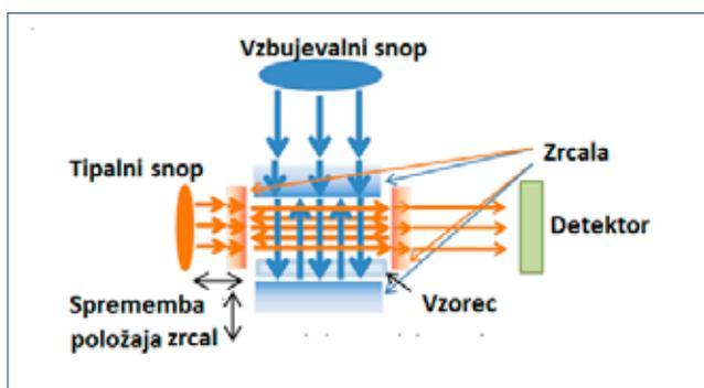
Geometry of the upgraded BDS system with microscopic optics and resonant cavity. The upgraded system was used for iron detection in passive samplers on the basis of the diffusion gradients in thin film (DGT) technique, in which Fe(II) and Fe(III) are bounded to ion exchange resin (LOD = 12 nmolL<sup>-1</sup>).
