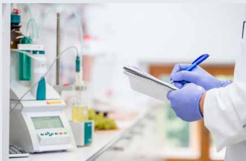
Measuring total titratable acidity in grape juice with automatic titrator.
