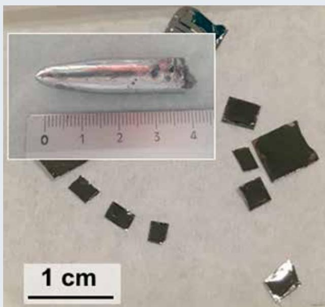
Layered  $\text{Bi}_2\text{Se}_3$  single crystals synthesized by the Bridgman method. The single crystal flakes were separated from the ingot shown in the insert.
