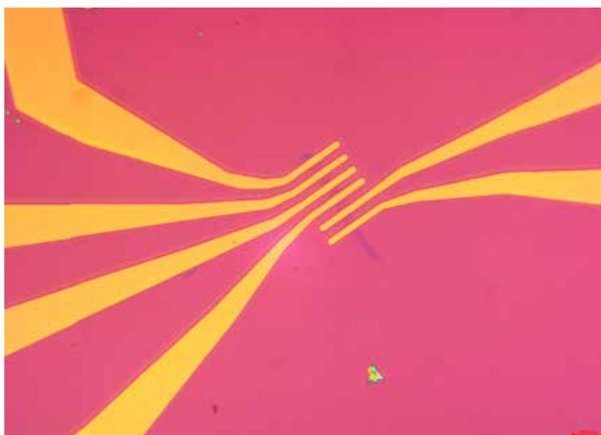
Optical micrograph of the single-layer graphene, obtained by the method of mechanical exfoliation from a bulk piece of graphite, on a silicon dioxide wafer and gold electrodes (yellow colour) on it, fabricated by means of laser lithography. The resulting graphene field-effect transistor was used to study charge transport properties of graphene.
