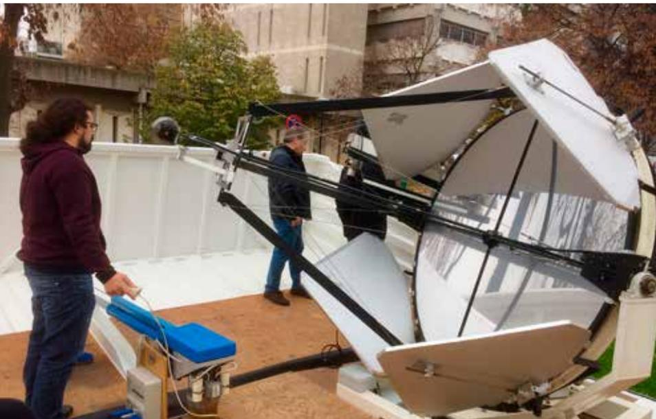
Center for atmospheric research team takes part in the development of the prototype of the Raman lidar for the Cherenkov Telescope Array (CTA) observatory. The lidar, which is being built at *Universitat Autònoma de Barcelona* (UAB), is required to provide atmospheric optical properties up to 20 km height in less than a minute.
