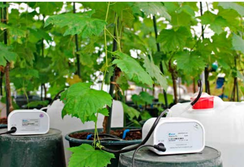
Pot experiment with vine plants irrigated with the tap water, with the treated model waste water, cleaned with electrochemical approach, and with the model waste water.
