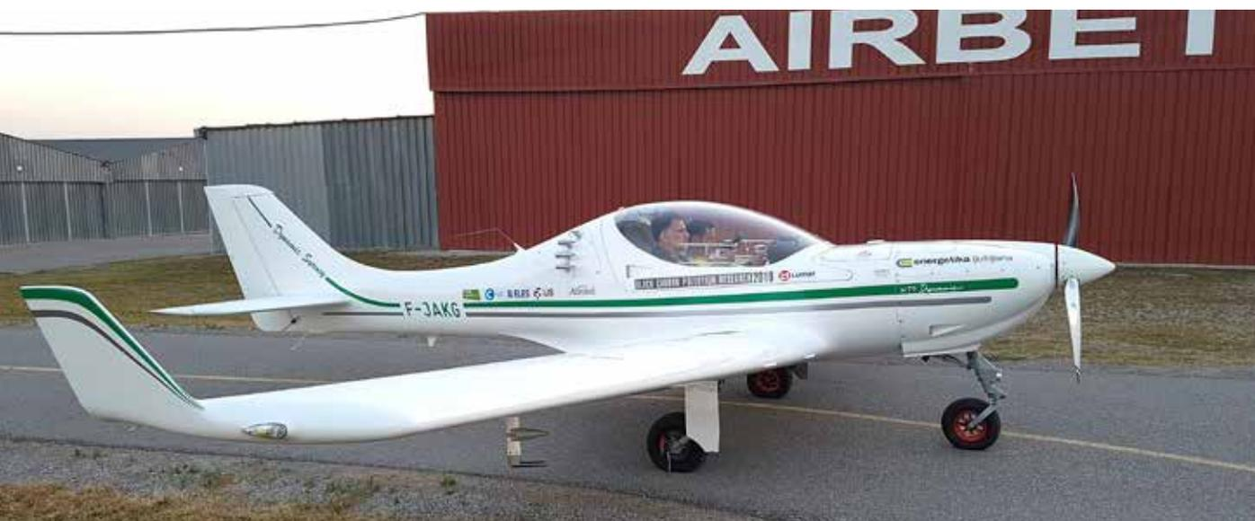
The aircraft with the equipment for measurement of pollutant vertical profiles. We see the fine aerosol inlet under the wing and the coarse aerosol inlets on the fuselage.
