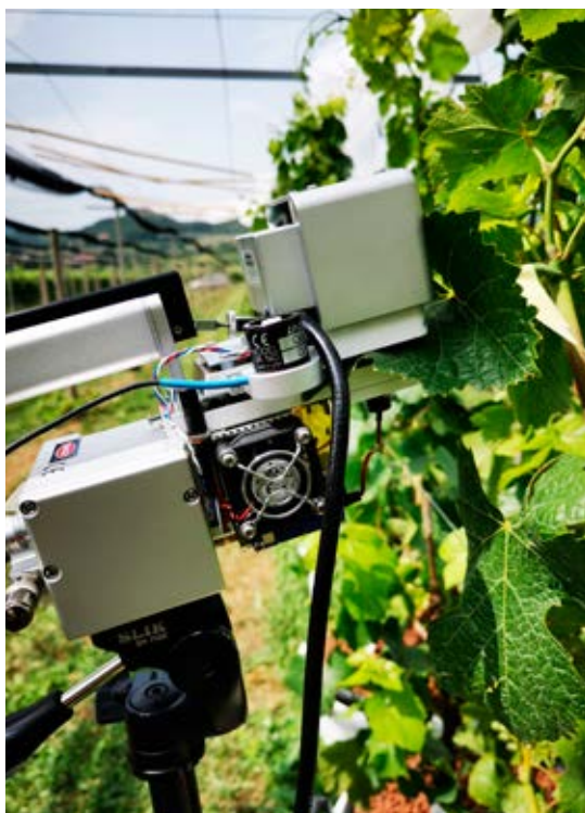
Measurement of grapevine leaf photosynthetic activity and stomatal conductance with an infrared gas analyzer (in cooperation with the Agricultural Institute of Slovenia).
